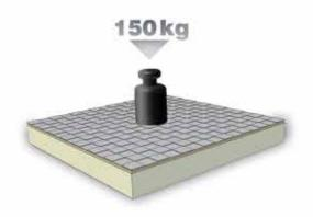
**Cold room floors** are sandwich type panels consisting of profiled galvanizeed metal sheet 1,25mm thick on the inner side which is coated with a PVC film 150 microns thick, and the polyurtethane filling with the galvanised metal sheet of 0,6mm thickness on the outer side. On the inside of the inner metal sheet we add the 12mm chipboard and only after that we fill it with polyurethane. In this way we get load-bearing capacity of the floor of 150kg/m2.
