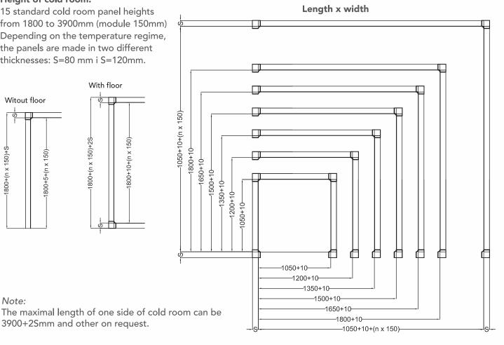
Inner dimension of the cold room = total length(width) of the panel +10External dimensions of the cold room = inner length(width) of the cold room +2S
