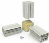
Cold room housing frame is separable construction consisting of PVC profiles and corner elements. It is specially designed for easy cleaning, and it satisfies the HACCP requirements.
